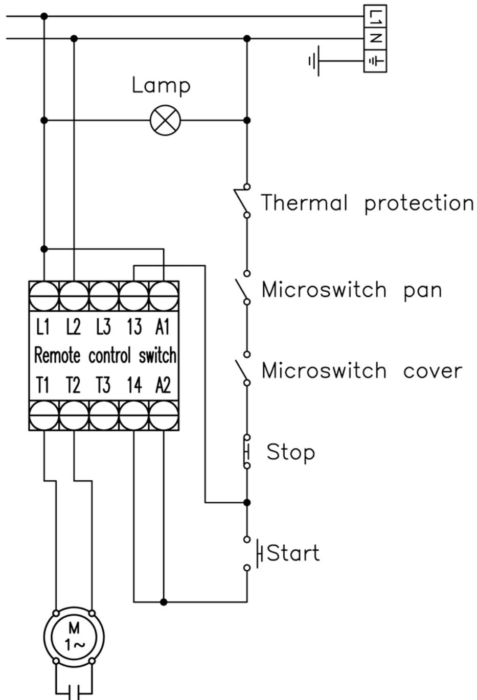
SCHEMA ELETTRICO • ELECTRICAL WIRING DIAGRAM •
